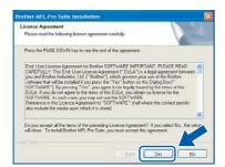
When this screen appears, connect the Parallel interface cable to your PC, and then connect it to the machine.
